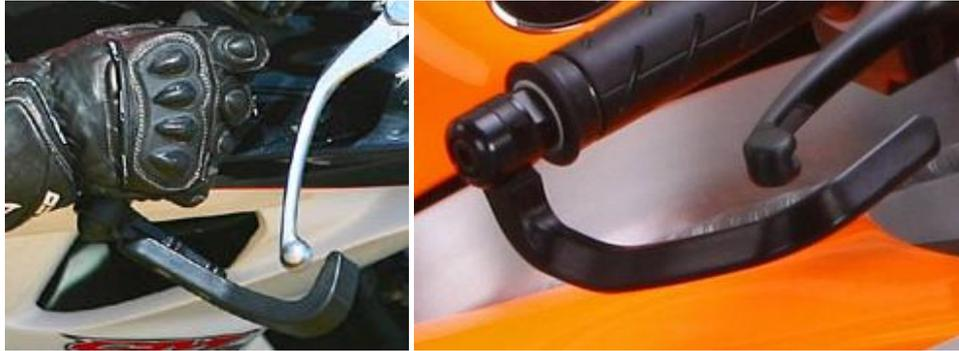
Picture 15 - Examples of front brake lever protections
