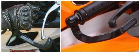
Picture 15 - Examples of front brake lever protections
