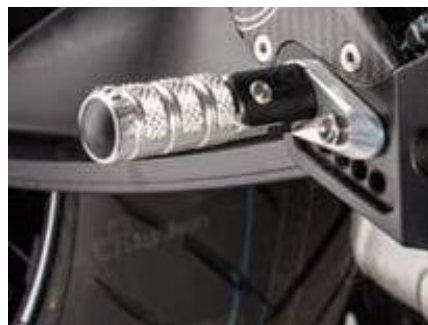
Picture 16 Footrest ends. Left, footrest with hole, not allowed; Right, footrest with cap, allowed.
